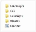
The releases folder does not exist initially. It is created as soon as an installer is made. The bake.bat batch file is the starting point of creating the installer. Double-clicking it will start the creation procedure. The three installers are stored in the releases folder. The bakescripts folder contains a couple of Python sources to initiate and support the creation. The nsis folder contains version 2.46 of NSIS and the nsisscripts folder the NSIS sources of HiSPARC.
